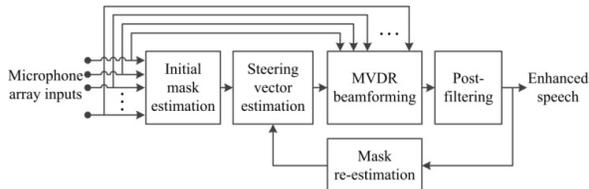
Fig. 1. Schematic diagram of the proposed speech enhancement algorithm.
