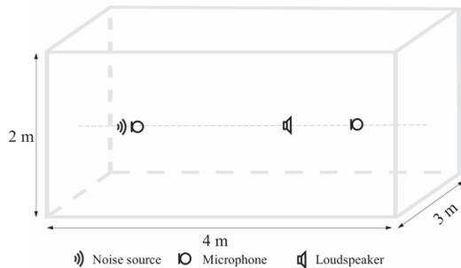
Fig. 7. Illustration of the ANC experimental setup.
