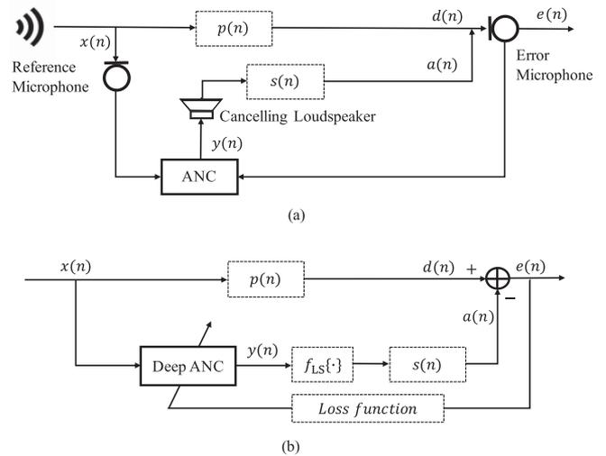
Fig. 1. Diagrams of (a) feedforward ANC system, and (b) deep ANC approach.
