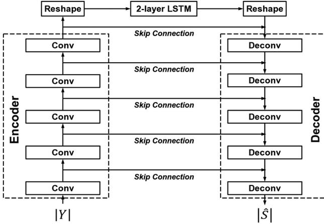
Fig. 2. Illustration of the CRN for spectral mapping in [32]. The CRN comprises three modules: An encoder module, an LSTM module, and a decoder module. ‘Conv’ denotes convolution and ‘Deconv’ deconvolution.
