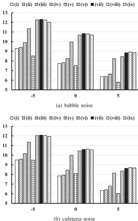
Fig. 6.  $\Delta$ SNR in dB over the unprocessed mixtures for  $-5$ , 0 and 5 dB. The approaches are (i) CRN + TMS [32], (ii) CRN-RI + TMS, (iii) GCRN + cIRM ( $G = 1$ ), (iv) GCRN + cRM-SA ( $G = 1$ ), (v) CNN + TCS [6], (vi) GCRN + TCS ( $G = 1$ ), (vii) GCRN + TCS ( $G = 2$ ), (viii) GCRN + TCS ( $G = 4$ ) and (ix) GCRN + TCS ( $G = 8$ ).
