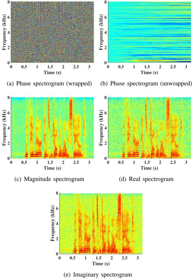
Fig. 1. (Color Online). Illustration of phase, magnitude, real, and imaginary spectrograms of a speech signal. The magnitude, as well as the absolute values of the real and imaginary spectrograms, is plotted on a log scale.
