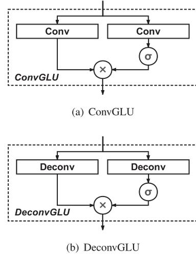
Fig. 3. Diagrams of a convolutional GLU block and a deconvolutional GLU block, where  $\sigma$  denotes a sigmoid function.
