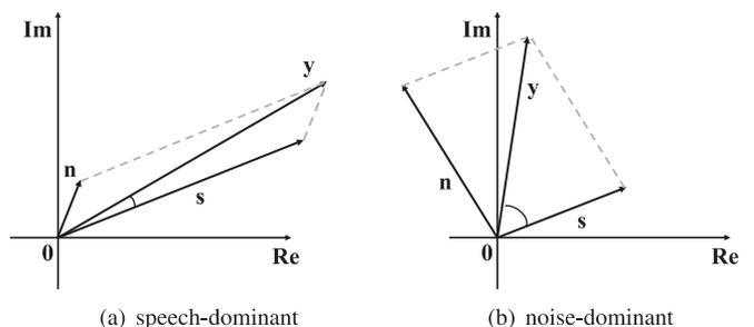
Fig. 9. Illustration of phase error under different conditions.
