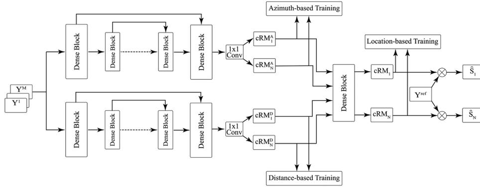
Fig. 2. Schematic diagram of the proposed joint training framework for location-based training.  $\text{cRM}_n^A$ ,  $\text{cRM}_n^D$  and  $\text{cRM}_n$  refer to the estimated complex ratio masks of the  $n$ -th speaker by the azimuth branch, the distance branch and the fusion model, respectively.
