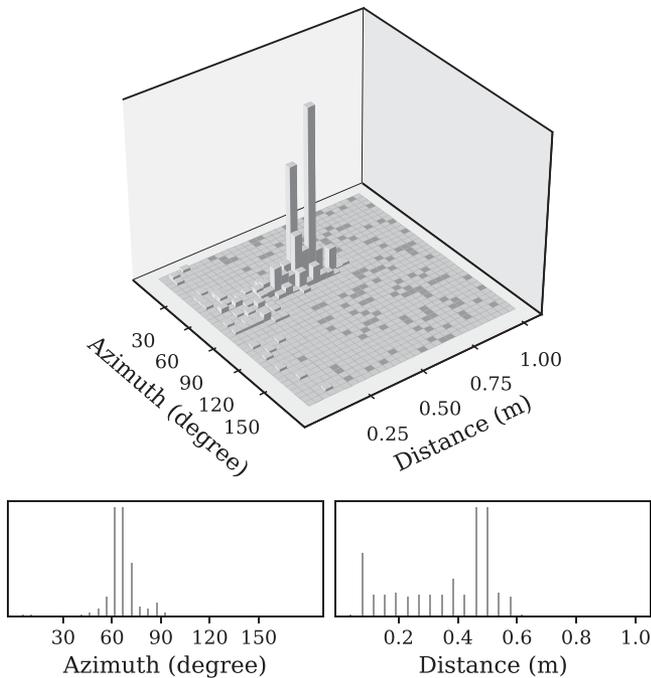
Fig. 4. Histograms of frame-wise estimated azimuths and distances for a 2-speaker mixture in a reverberant room with  $T_{60}=640$  ms. Speaker distances from a 7-channel microphone array are 0.43 m and 0.50 m and azimuths are  $60^\circ$  and  $65^\circ$ .
