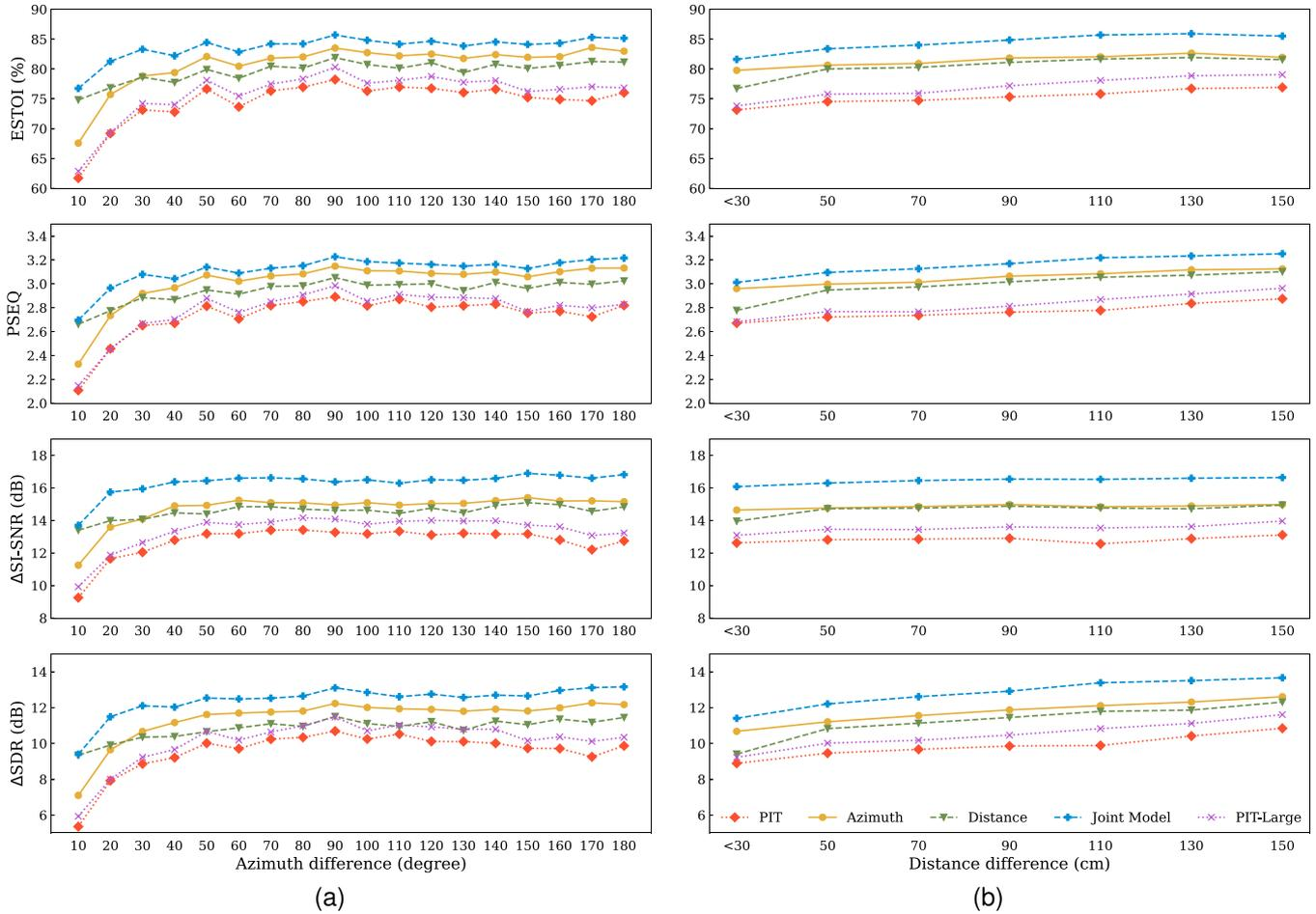
Fig. 3. Average results on reverberant 2-speaker mixtures with the 7-channel array, based on (a) azimuth difference with  $10^\circ$  intervals and (b) distance difference with 20 cm intervals. ‘PIT-Large’ refers to the PIT-based MC-CRM model with a larger number of parameters.
