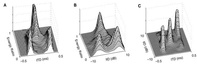
Figure 1: A: Relationship between ITD and the energy ratio. B: Relationship between IID and the energy ratio. C: Clustering in the ITD-IID feature space. Histograms are obtained for speech at 0° and interfering noise at 30° and -30°, for the channel number 85 with center frequency ~1.7 kHz.
