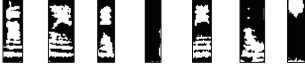
Fig. 1. IBMs of phones /aa/, /ae/, /eh/, /h#/ (sil), /iy/, /ow/ and /s/, ordered from left to right. In the figure, a white pixel indicates 1 and a black pixel 0. Note how the IBM captures the high energy regions of the phone (none for silence).
